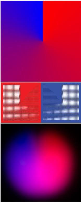
**Figure 3:** Top: A red/blue circular gradient target image, input to our system. Middle: The red and blue cut gel patterns our system outputs. Bottom: The lit result of the gels affixed to a conventional fixture.
