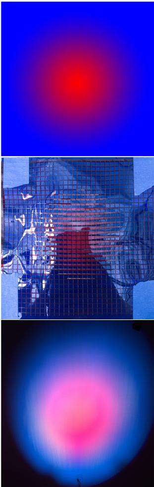
**Figure 5:** Top: Target image of a red center and blue background. Middle: The corresponding layered gels taped on a gel frame. Bottom: The lit result of the above gels.
