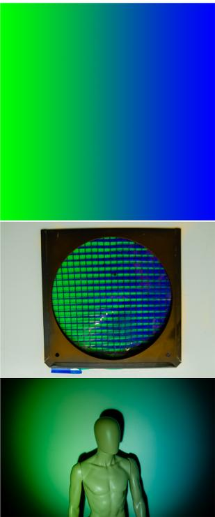
**Figure 2:** The entire process of designing a blue/green gradient gel. Top: Target image. Middle: Cut gels in a gel frame. Bottom: The lit result on a human-sized mannequin for scale.
