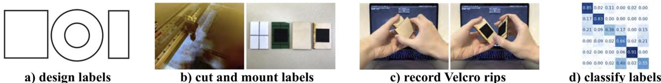
Figure 1. Our acoustic labeling process comprises a) designing label shapes using a SVG editor b) cutting the labels from the paired sides of Velcro strips and attaching them to surfaces c) recording the sound generated by separating the two sides d) classifying the labels based on their audio signal.
